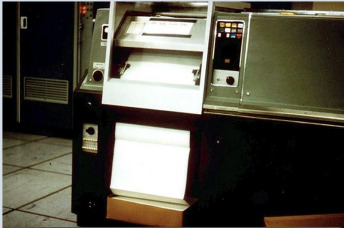
Anelex printer – which could be modified to produce raised dots for Braille readers
