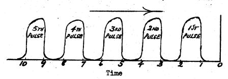
If now the pattern of these pulses is made to correspond to the "l"s and "0"s of a binary number, that number can be used in the machine in the form of a pulse train.
