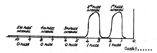
This is again the binary from of E; a pulse represents "1", and the absence of a pulse in a position where a pulse may occur represents "0".
