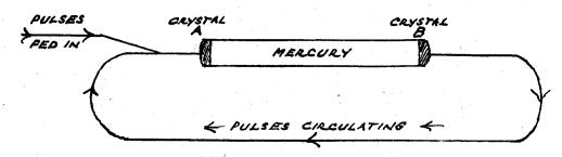
When a circulating pulse arrives at crystal A, the crystal sets up a vibration in the mercury which travels to crystal B. At crystal B this vibration sets up an electrical pulse which travels along the wire to crystal A again, and so on.
