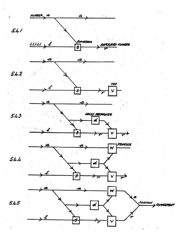
The additional pulses may be made available by connecting to the feed line a lead,  $\ell$ , which carries a continuous pulse-train lllllllll (see figure 5.5.2.). But this continuous pulse-train must not be allowed to disturb the partial product flowing from the Multiplicand circuit until the Negative Digit position has arrived; a tap  $\underline{\mathbf{v}}_i$  must therefore be interposed to block them (see figure 5.5.3.).
