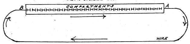
As the pulses included in each compartment pass along the wire A B to re-enter the Delay Storage mechanism, the information they convey may be read off for use by the machine. Also when fresh information is required to be stored, it can be put in the appropriate compartment as it passes along the wire.
