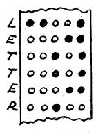
To put information into the Machine, punched tape is first preduced in this way whether the information consists of numbers, orders, or letters. Numbers, orders and words are typed into the Punch just as into a typewriter.
